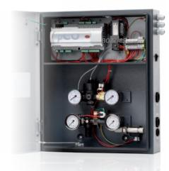
The system uses compressed air to atomize the water into very fine droplets that evaporate spontaneously in the air, humidifying and cooling it. The electronic controller manages the water and compressed air supply to the nozzles, plus all the automatic cycles, such as nozzle cleaning and washing.
