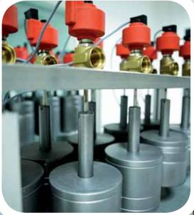
CAREL E<sup>x</sup>V valves have been lifetime tested in the **most critical** operating conditions by the CAREL labs
