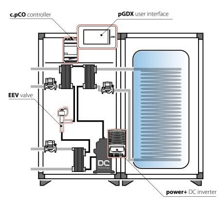
The software has been designed on the c.pCO programmable controller platform:
