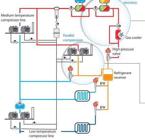
Heat recovery parallel compression focus inside a typical installation scheme (Transcritical CO, booster system)
