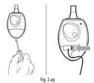
The functions are selected by setting the two dipswitches, accessible by removing the battery cover.
