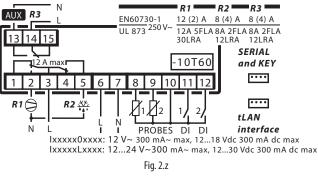
Thermostats with 3 relays: compressor, defrost, evaporator fans
