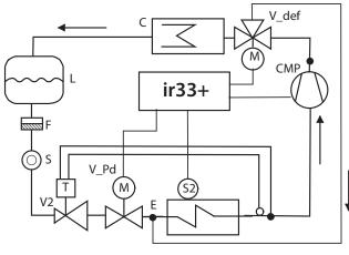
**Note:** the defrost output (DEF) is used to control the hot gas valve V def.
