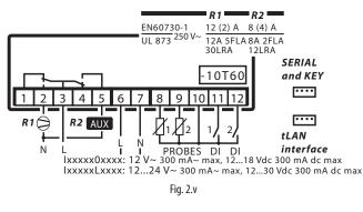
Thermostats with 2/3 relays: compressor, defrost, AUX
