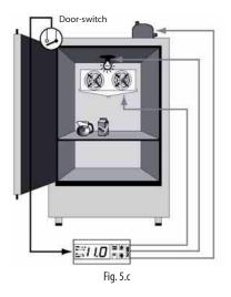
Note: if more than one digital input is configured as a door switch, the door is considered open when at least one of the inputs is open.
