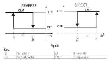
If the second compressor output is activated (H1, H5 = 12) on the AUX output, the compressor output is activated at  $St\pm rd/2$  and the AUX output at  $St\pm rd$ , as illustrated in the following figure.
