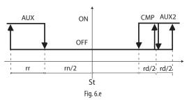
Reverse operation (r3 =2), with 1 compressor output (CMP) and 2 compressor outputs (CMP and AUX2).
