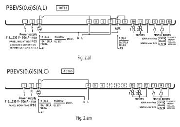
Thermostats with 2/3 relays: compressor, defrost, AUX
