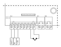
**Fig. 4.k** CAREL NTC probe connection:
