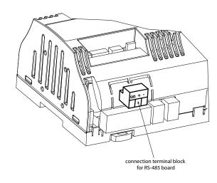
Fig. 5.d (detail of the electronic board, humidifier electrical compartment)
