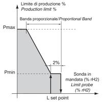
Fig. 14.3 Control with limit probe
