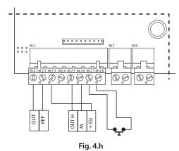
The reference (zero) of the external controller must be connected to the GND terminal (M2.2) and the control signal to terminal M2.1 CONTROL WITH CAREL MAIN PROBE
