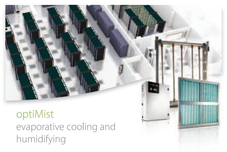
optiMist is an evaporative cooler and humidifier that atomises water in fine droplets which, while spontaneously evaporating, remove heat from the humidified and cooled air. It uses a vane pump to pressurise the water, subsequently atomising it through special nozzles.
