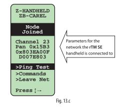
In both cases, press the "Up" and "Down" buttons to scroll the menu; press the "Right" button to activate the selected function.
