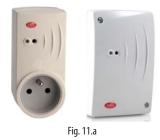
The rTM wireless Plug and Switch devices are modules with the same features and are proposed with different electrical connections for adaptation to specific requirements. They comprise an energy meter and a control relay that can handle up to 2.5 kW single-phase electrical loads. These devices are installed between a normal 230 Vac power socket and the load being controlled.
