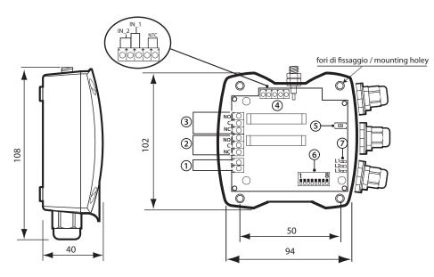
12... 24 Vac/dc power supply; 2-3 SPDT relay output;
