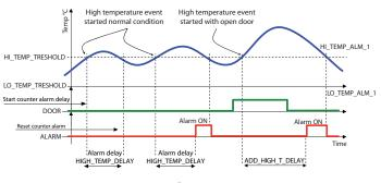
The figure shows the high temperature alarm function:
