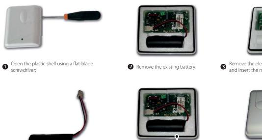
Insert the new battery codeWS00BAT200 and 4 connect the connector, observing the correct polarity;
