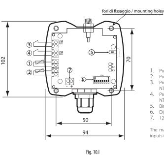
1. Pulse counter digital input 1 (IN\_1); 2. Pulse counter digital input 2 (IN\_2);
