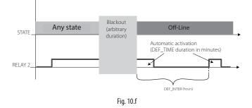
**Note:** starting from firmware version 2053, the activation of Relay 2 (defrost relay) causes the consequent deactivation of Relay 1 (control relay).
