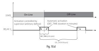
Behaviour of Relay 2 on reset: the device saves the state of the defrost relay to non-volatile memory, consequently an off/on cycle does not change state.
