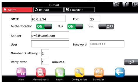
The screenshot displays the 'E-mail' configuration page. At the top, there are tabs for 'Alarm' and 'Guardian', and a 'Reload' button. The configuration fields are as follows:
