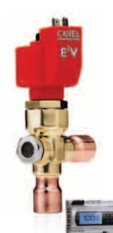
Modulation of refrigerant flow quarantees a wide operating range, due to the combination of the fixed opening and the moving element with a travel of 15 mm driven by stepper motor.
