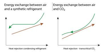
Condensation normally takes place at constant pressure, with the gas changing to the liquid phase, while in a transcritical cycle, the temperature of the supercritical gas falls constantly.
