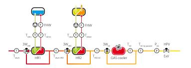
Heat recovery management allows complete control of two heat exchangers and related circulating pumps (in the case of  $CO_2$ -water) Activation and control of each heat recovery cycle is based on the percentage of heat demand, calculated using one of the following:
