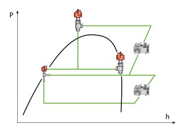
The HPV valve control algorithm on pRack pR300T is managed based on the gas cooler outlet temperature TGC and gas cooler pressure PGC. Depending on operating conditions, the system can work in:
