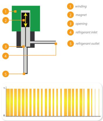
Diagram of the operating principle of a generic PWM expansion valve. PWM valves can only achieve a variation in the "average flow" over a period of several seconds. Instant flow can only be 100% or 0%.
