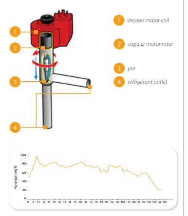
Diagram of the operating principle of a generic proportional expansion valve. The main plus of CAREL E<sup>2</sup>V proportional valves is axial rather than rotary movement of the control pin. Stepper valves can precisely and continuously modulate refrigerant flow based on the quantity needed by the system at any given time.
