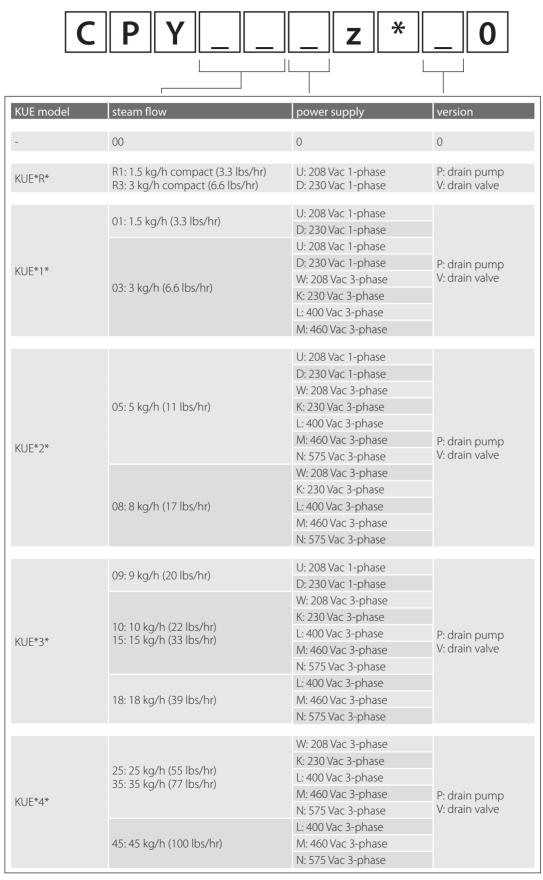
blank to be configured by humiSet, the CAREL kit for configuring the controllers, by CPYTERM or via network.
