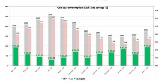
It is evident how the energy consumption values fluctuate during the whole year, due to the external temperature modifications (and since temperature inside the cold room is kept at a fixed -20°C).
