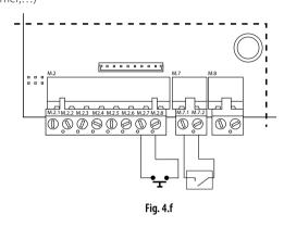
2. Enable and control the steam production using:
