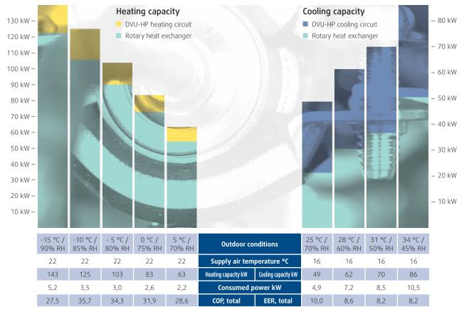
Performance example: DV 40 with 2,5 m<sup>3</sup>/s. Extract 22 °C/35% RH. Defrosting is not taken into account.
