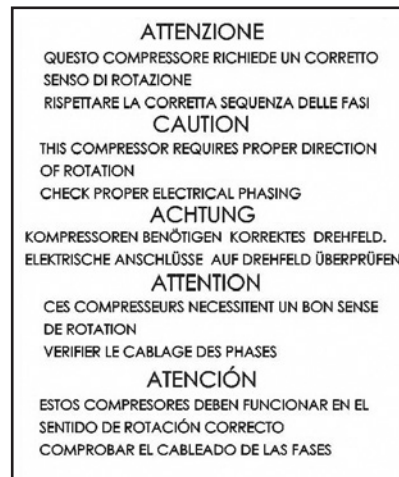
Sequence phase control on the electrical board
