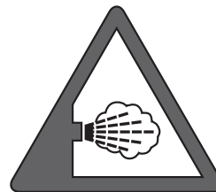
Warning - safety valves' vents
